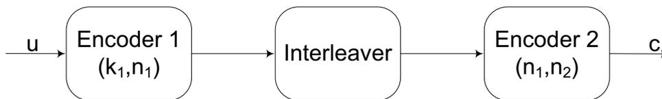
**Fig. 2.6** Serial Concatenated Block Code Encoder
