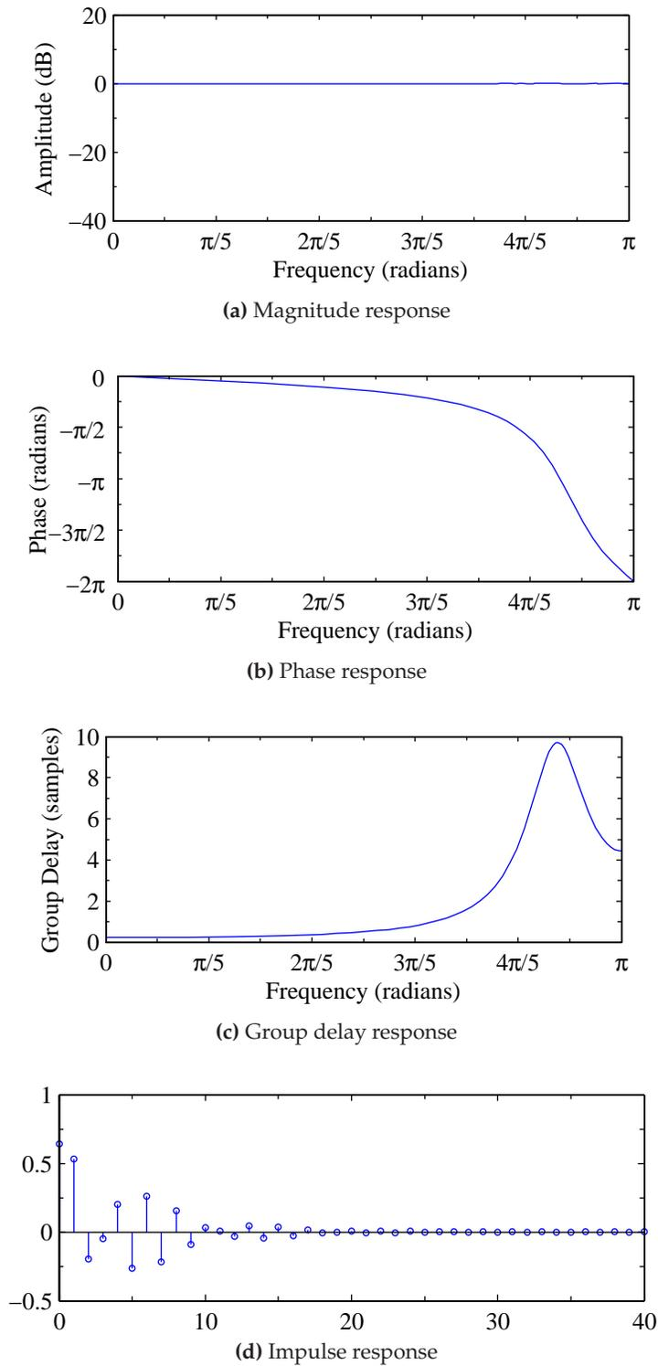
Fig. 6 Frequency and impulse responses of the all-pass filter.
