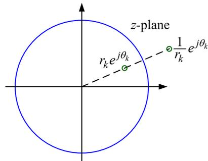
**Fig. 1** Zero symmetries: reciprocal zeros at  $z_k$  and  $1/z_k^*$ .
