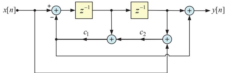
Fig. 3 Second-order all-pass structure using a minimum number of multiplies.
