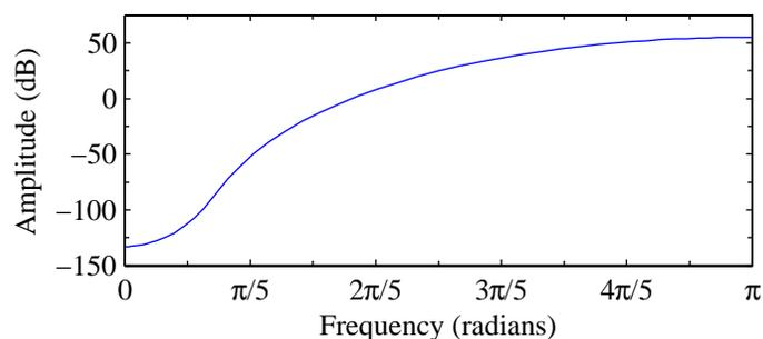
**Fig. 10** Amplitude response for a filter with minimum-phase zeros.
