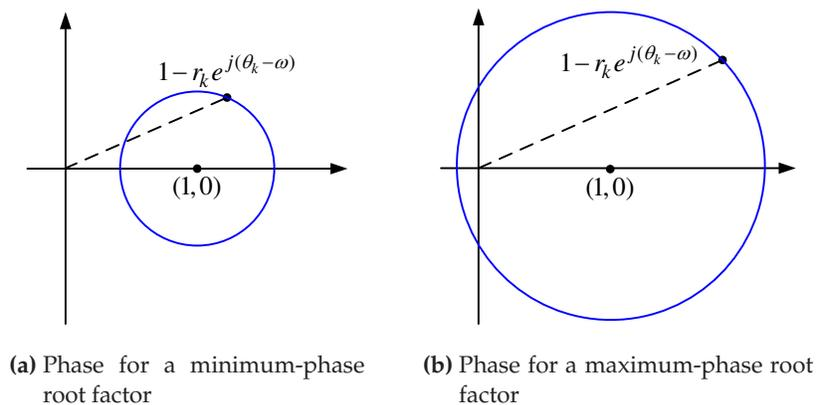
Fig. 2 Illustrating the phase of a root factor in the complex plane.
