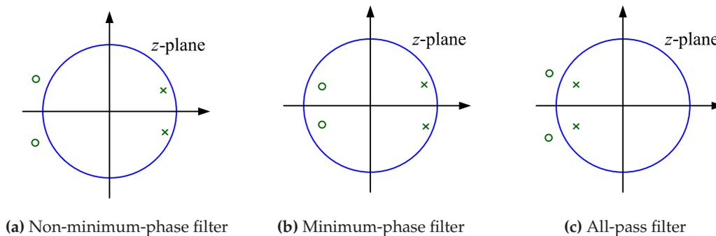
**Fig. 4** Pole/zero plots for the decomposition of a non-minimum-phase filter.
